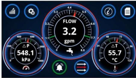
Essentially, the greater the flow the more cooling you achieve. To get maximum flow, the goal is to achieve turbulent flow. In this state the water molecules are 'bouncing' off of the sides of the pipe meaning more effective heat removal of heat from the mould. The measurement of flow is known as a Reynolds (Re) number and this number can be displayed in the centre of the flow dial
