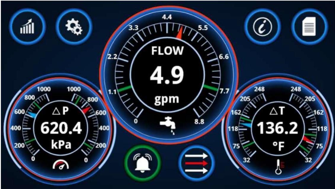
This view is available if both a Flow sensor and a Pressure sensor is connected to the system. Depending on the sensor type connected, you will either be able to see Flow, Pressure, Temperature and Delta T, or Flow, Pressure, Delta P, Temperature and Delta T.
