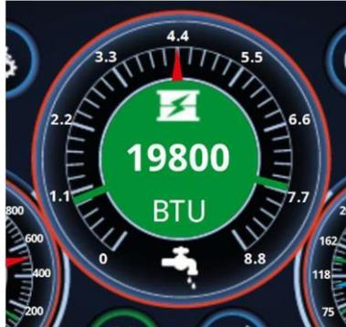
By Pressing the Centre of the Flow Dial the display will cycle between Flow, Reynolds Number and Energy (only available on Double Sensor Installations).
