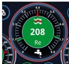
The calculation is based on the diameter of the flow channel and the amount of glycol within in the system; these parameters can be changed on the settings page.
