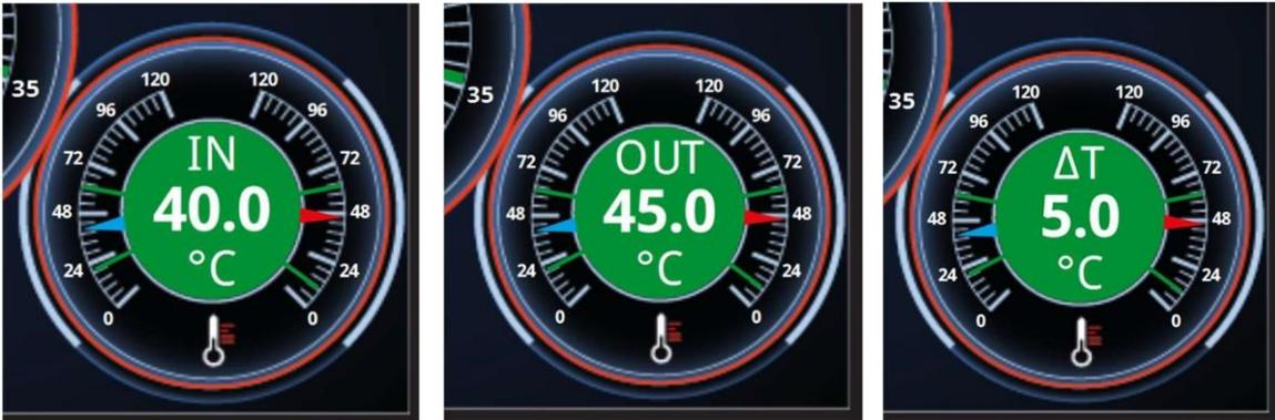
By Pressing the Centre of the Temperature Dial the display will cycle between Temperature IN, Temperature OUT and Delta T (only available on Double Sensor Installations).
