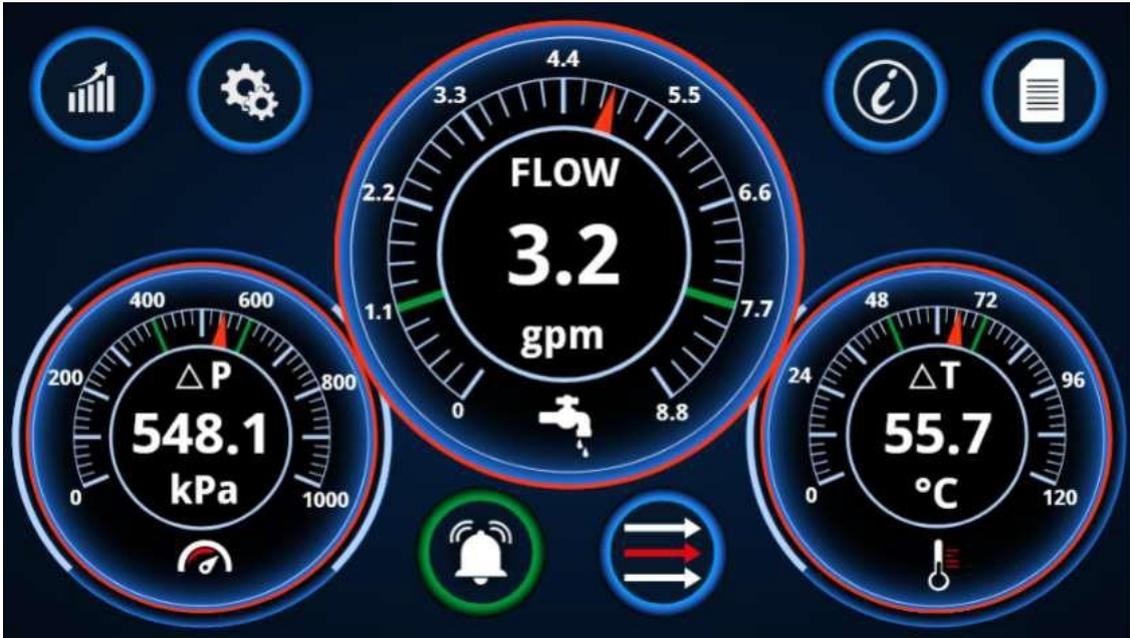
This view is available if only a single sensor is connected to the system. Depending on the sensor type connected, you will either see Flow & Temperature or Flow, Temperature and Pressure.
