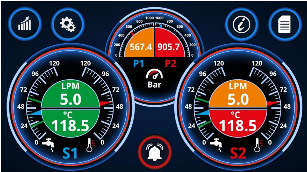
This view is available if both of the connected sensors are Flow sensors. Depending on the sensor type connected, you will either be able to see Flow and Temperature or Flow, Temperature and Pressure.
