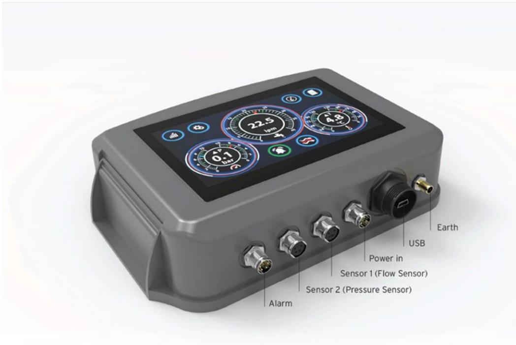
Note : If you notice erratic readings on the screen there may be noise on the sensor signal then connect an earth cable between the Earth stud on the FloSense unit and a hard earth reference point on the pipework.
